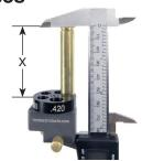
X = relative measurement between the base of a case to a datum point on its shoulder angle.
