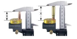
X = relative measurement from the base of a bullet/cartridge to a point on the bullet's ogive, very close to the bullet's major diameter.
